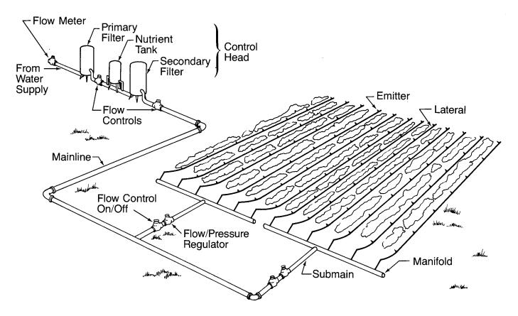
Trickle irrigation which is diagramed here, conserves water by getting most of it to the roots and keeping the surface relatively dry. It is suited for valuable, widely spaced crops like trees or vines.
