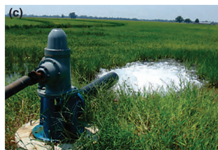
Irrigation well used for flood irrigation of a rice field in the Mississippi Delta region. (Photo by David E. Burt, Jr., USGS)
