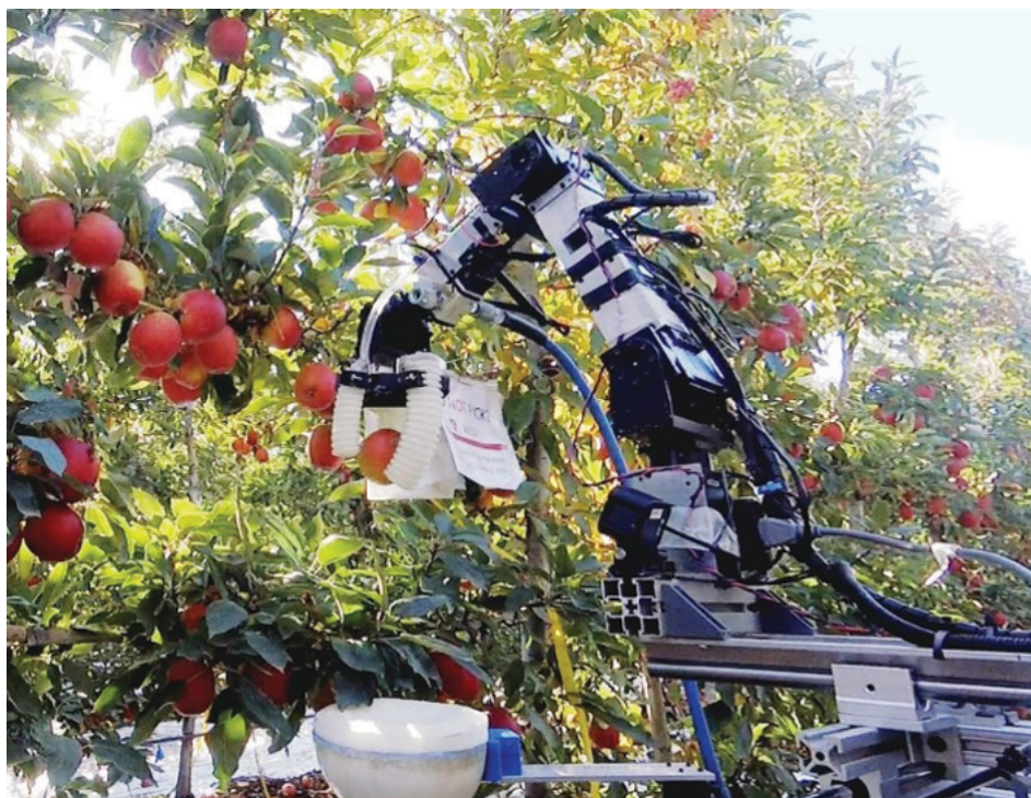
Figure 6. Apple Harvesting Robot. (Photo Credit: Manoj Karkee, Washington State University.)
