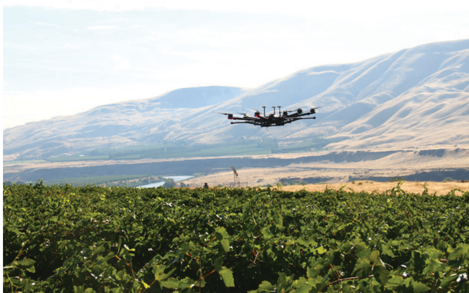
Figure 7. UAS used for automated bird pest deterrence in vineyard. (Photo credit: Manoj Karkee, Washington State University.)
