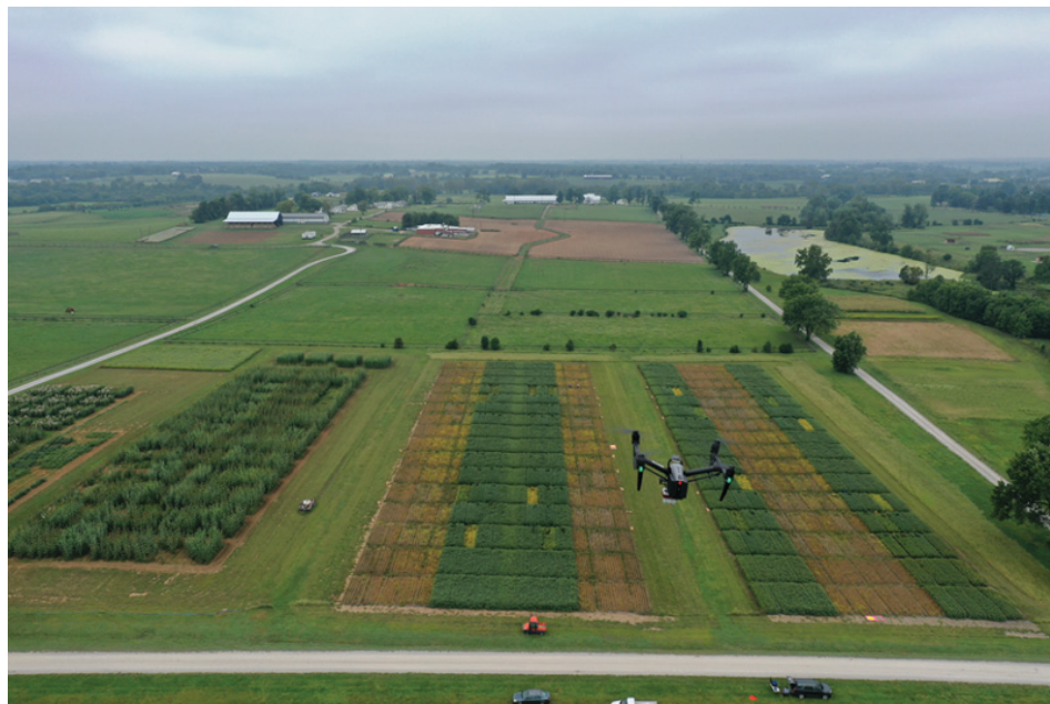
Figure 5. A Multirotor UAS collecting multispectral images of soybean plots. (Photo Credit: Michael Sama, University of Kentucky.)
