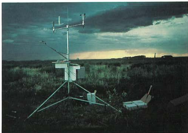
Figure 7.2. Automated weather station used to collect weather data for use in scheduling irrigations and other farming operations. Photograph courtesy of Dr. K. G. Hubbard, High Plains Regional Climate Center, University of Nebraska, Lincoln.
