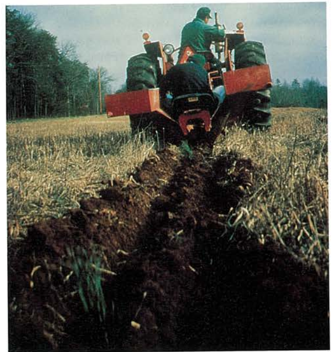
Figure 1.3. Tree planting machines used to plant tree seedlings, such as these Loblolly pine trees ( Pinus taeda L.), on most agricultural land. Photograph courtesy of Robert J. Moulton, USDA, Forest Service, Washington, D.C.
