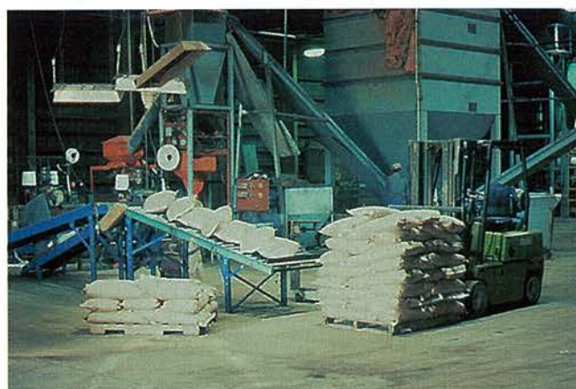
Figure 5.1. Commercial processing of poultry litter into cattle feed. Photograph courtesy of Thomas A. McCaskey, Auburn University, Auburn, Alabama.
