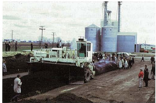
Figure 5.3. Mechanical mixing of composting cattle manure. Photograph courtesy of Don D. Jones, Purdue University, West Lafayette, Indiana.
