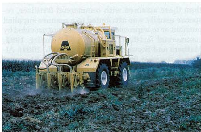
Figure 4.2. Incorporation of liquid manure into the soil. Photograph courtesy of Alan L. Sutton, Purdue University, West Lafayette, Indiana.
