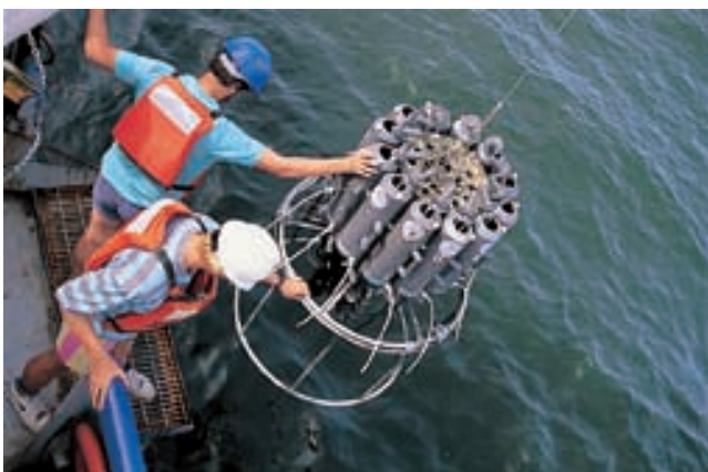
Figure 2.4. Deploying conductivity, salinity, temperature, dissolved oxygen, and depth (CTD) meter in hypoxia research. Photograph by Franklin J. Viola, Viola Photo Visions, Inc., Roswell, Georgia.
