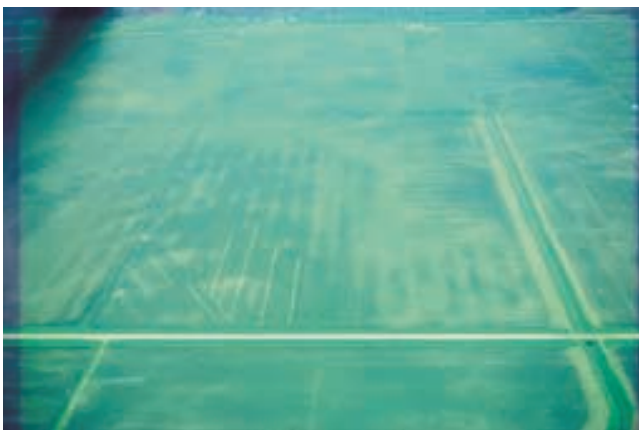
Figure 4.3. Aerial photograph showing drainage patterns of farm fields in Central Iowa. The light, straight lines in the wet field are areas where tile drains have removed subsurface water. Photograph courtesy of Dr. James L. Baker, Iowa State University, Ames, Iowa.
