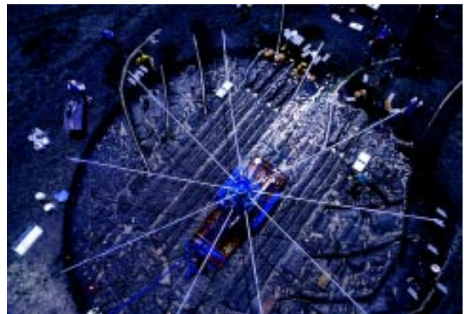
Figure 4.2. The rainfall simulator and test plot at Cottonwood, South Dakota, enabled technicians to measure water runoff rates and collect soil samples in a Water Erosion Prediction Project cropland field study. Photo courtesy of T. McCabe, Agricultural Research Service, U.S. Department of Agriculture, Beltsville, Maryland.
