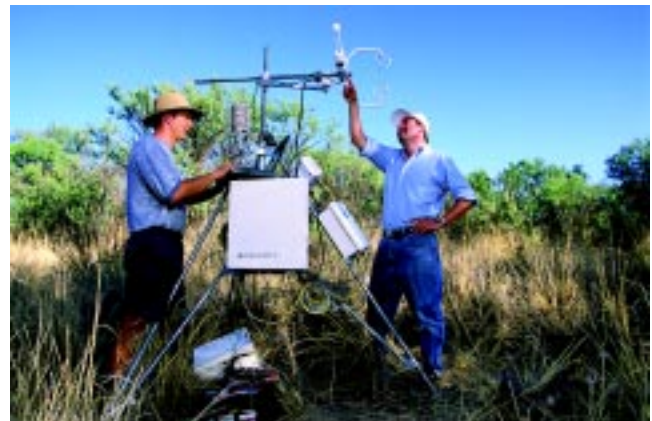
Figure S.4. Researchers from the University of Arizona download data from a meteorology/flux system that measures the amount of water and C exchanged among vegetation, soil, and atmosphere. Photo courtesy of P. Greb, Agricultural Research Service, U.S. Department of Agriculture, Beltsville, Maryland.
