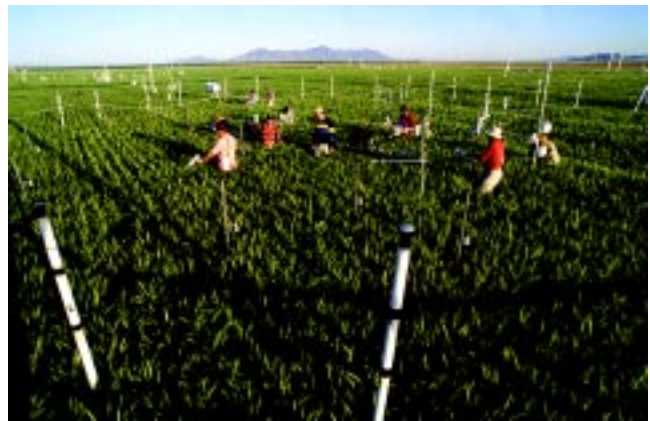
Figure 1.7. Scientists measure the growth of wheat surrounded by elevated levels of atmospheric CO 2 near Phoenix, Arizona. The study, called the Free Air Carbon Dioxide Enrichment, is to measure CO 2 's effect on plants. It is the largest experiment of this type ever undertaken. Photo courtesy of J. Dykinga, Agricultural Research Service, U.S. Department of Agriculture, Beltsville, Maryland.
