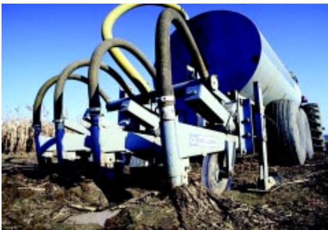
Figure 2.14. Manure injection on a farm in Maryland. Photo courtesy of T. McCabe, U.S. Department of Agriculture.
