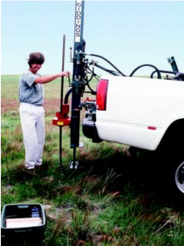
Figure 4.1. Hydrologic probe equipment such as this is used routinely to extract soil cores that then are taken to the laboratory for processing and measurement of C content. Photo courtesy of S. Sprague, Colorado State University.
