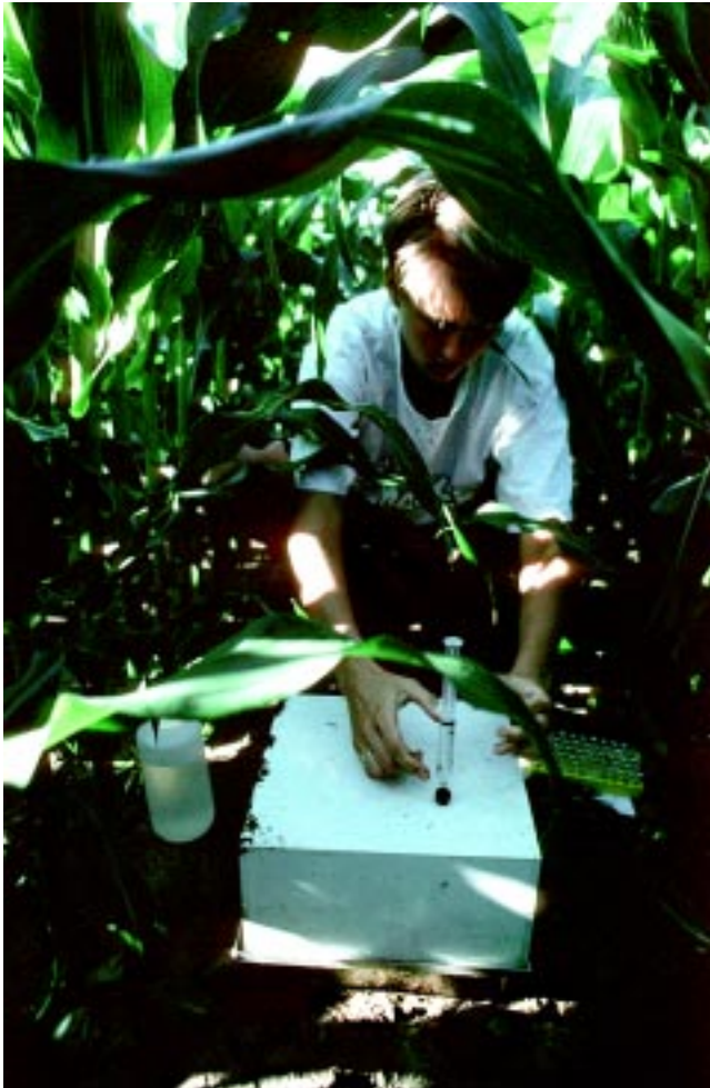
Figure 4.5. A static flux chamber measurement being taken in a growing corn crop. Typical designs use a removable cover that is placed on a semipermanent base (can be removed for tillage) having an airtight seal. For soil trace gas measurements, the area within the chamber usually is kept vegetation-free to eliminate \text{CO}_2 uptake by plants. For measurements, the cover is sealed and left for several minutes to allow the gas being measured to accumulate in the chamber (or to be consumed where there is uptake by the soil), and a series of gas samples are taken via syringe (for later analysis on a gas analyzer) to determine the change in gas concentration over time, from which flux rates are determined. Photo courtesy of G. P. Robertson, Michigan State University.
