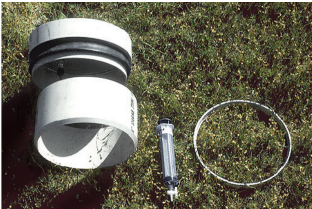
Figure 2.6. Example of a polyvinyl chloride (PVC) chamber used by GRACenet research for measuring emissions/exchanges of greenhouse gases from the soil. The soil anchor (bottom left) is inserted permanently to a near surface level (right side). The chamber (top left) is attached to the anchor during the time that air samples are being collected using a syringe. Gas samples are subsequently analyzed using a gas chromatograph (Parkin and Venterea 2010).
