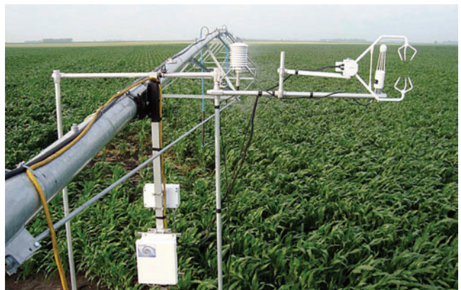
Figure 2.8. Eddy covariance system measuring \text{CO}_2 and \text{H}_2\text{O} fluxes above an irrigated corn field. The net upward and downward components of wind are measured by sonic anemometers at the extreme right of the apparatus (Baker and Kimball 2010).
