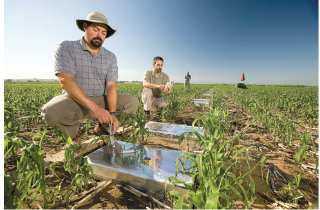
Figure 2.7. Example of a rectangular chamber being used by ARS technicians to measure emissions of greenhouse gases from soil in a field of corn at the Ft. Collins, Colorado, research location. (Photo courtesy of Stephen Ausmus [D1535-8].)
